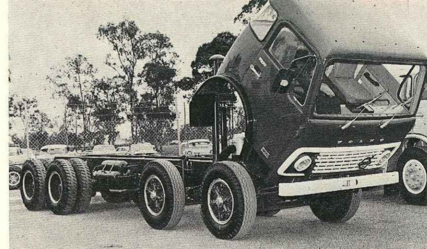
FIRST twin-steer Volvo model in the world is the Queensland-produced F86 8 x 4 (left), of which 15 have been ordered by Brambles. Australian content is 50%; front wheels, chassis frame rails, rear bogie and suspension as well as the braking equipment, fuel tank, etc., come from local suppliers.
