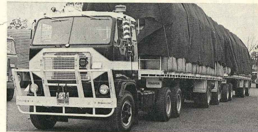
ROAD TRAIN make-up for a G88 6 x 4 (below) feature a Haulmark spread tandem 36 ft. semi plus an 8-wheel 36 ft. dog trailer. This prime mover, part of the display at the opening of Volvo's Wacol (Qld.) factory last month, had a heavy duty rear axle, Hendrickson suspension, 16-speed transmission.
