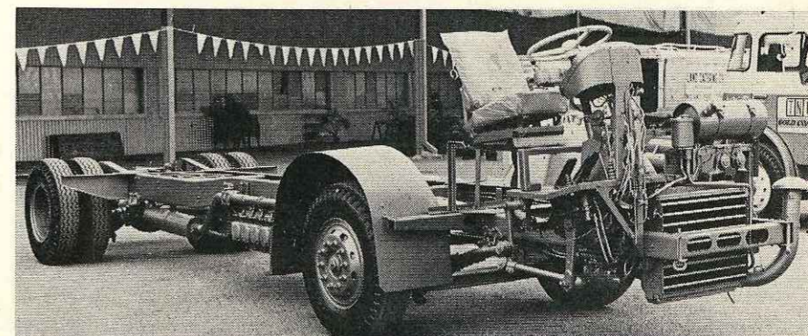
PRIOR to delivery to the well-known Grafton, NSW, hauliers Cromack Tranter, this G88 4 x 2 (above) went on display at Volvo's new assembly plant. BUS CHASSIS production at Wacol is confined to the B58 (below) and the B57 at the moment. The heavy duty B59 will come later. The model shown has 185 bhp normally-aspirated engine and electro-pneumatic transmission.
